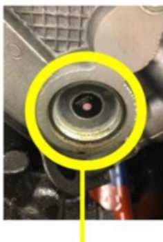
Overheated Pink Sensor 255°F Coolant Temp
