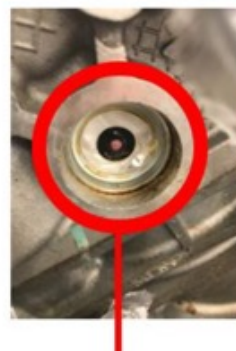
Overheated Red Sensor +255°F Coolant Temp
